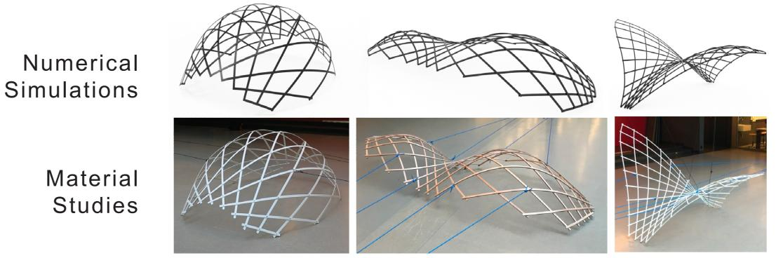
We performed material tests to characterize the strength of our GFRP beams, connector sleeves, and rivets. We also ran a detailed finite element analysis on the regions where our simulation algorithm predicted high beam stresses and forces on the joints. These experiments confirmed the robustness of our pavilion design.
