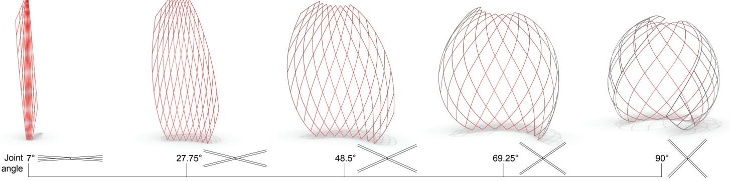
We deploy the pavilion simply by stretching it open: its curved 3D shape is encoded directly into the flat design, and the shape is robust to imprecision in the deployment process. Our pavilion does not require boundary supports to maintain its shape.
