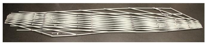
We build the pavilion in a perfectly flat state by connecting its beams with pivot joints.
