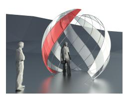
The X-Shell Pavilion is a lightweight structure composed of elastic beams joined in a special layout optimized for easy assembly and on-site deployment.
